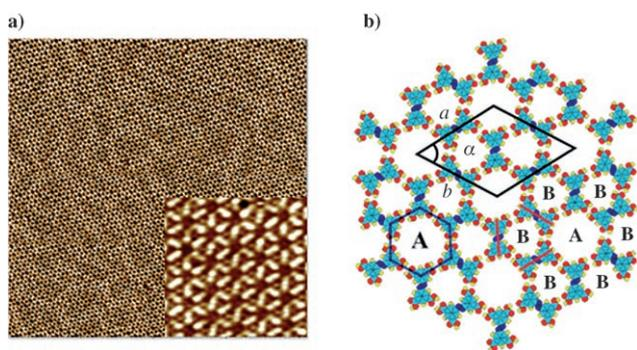
**Figure 2.** a) Constant-current STM image ( $103 \times 103$  nm) of a self-assembled monolayer of NN4A networks on highly ordered pyrolytic graphite (HOPG) surface.  $I = 549$  pA,  $V = 540$  mV. Inset: High-resolution view showing the detailed NN4A network structure. b) Proposed molecular model for the NN4A networks.
