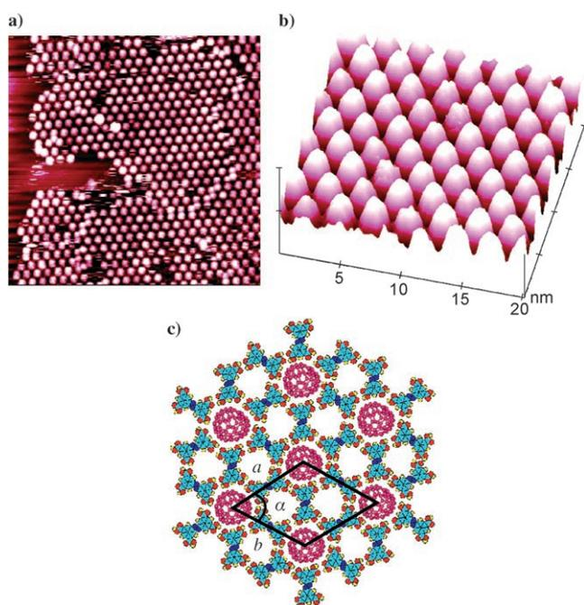
**Figure 4.** a) STM image ( $67.4 \times 67.4 \text{ nm}$ ) of the  $C_{80}$ -NN4A host-guest architecture on an HOPG surface.  $I = 169.5 \text{ pA}$ ,  $V = 918.5 \text{ mV}$ . b) High-resolution STM image ( $20.1 \times 20.1 \text{ nm}$ ) of  $C_{80}$ -NN4A assembled structure.  $I = 169.5 \text{ pA}$ ,  $V = 918.5 \text{ mV}$ . c) Plan view of the proposed structural model.
