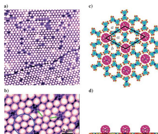
**Figure 5.** a) STM image ( $68 \times 68 \text{ nm}$ ) of the  $\text{Sc}_3\text{N}@C_{80}$ -NN4A host-guest architecture on an HOPG surface.  $I = 165 \text{ pA}$ ,  $V = 1008 \text{ mV}$ . b) High-resolution STM image of the  $\text{Sc}_3\text{N}@C_{80}$ -NN4A structure.  $I = 218 \text{ pA}$ ,  $V = 916 \text{ mV}$ . The green arrows indicate individual cavities missing one  $\text{Sc}_3\text{N}@C_{80}$  molecule. c) Plan view of the proposed structural model. d) Side view of the model.
